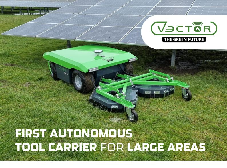
Vector machines is the specialist in autonomous (mowing) tool carriers for areas between 10ha and 100ha. Our A.I. driven software combines GPS, RTK and Lidar for accurate navigation on places with limited GPS coverage, such as solar parcs or under trees.
